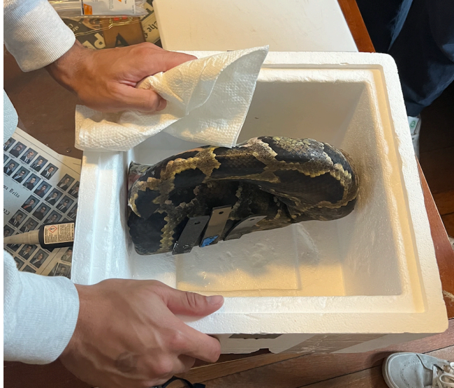
Figure 34. Strips with adhesive attached to our python sample before our force gauge lap shear testing.
