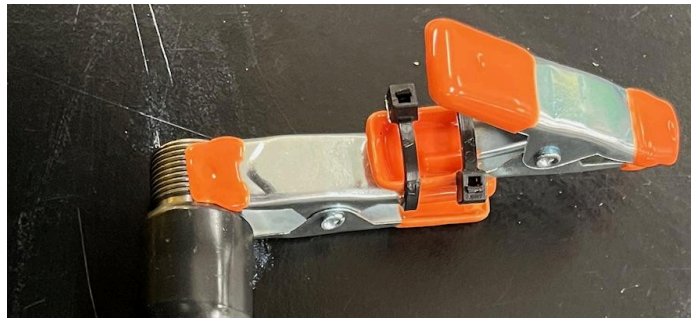
Figure 59: Image of double spring clamp connected together via a zip tie. The image also shows how the clamp connects to the male threaded rod end of the positioning arm.
