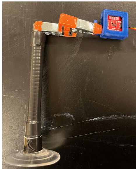
Figure H.9: Positioning arm and suction cup with the double spring clamp connected to the male end of the positioning rod and the clip of the sensor housing case.
