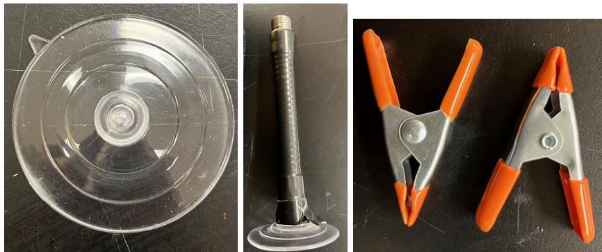
Figure H.6: Left to right: Suction cup, suction cup and positioning rod, and the double spring clamps.
