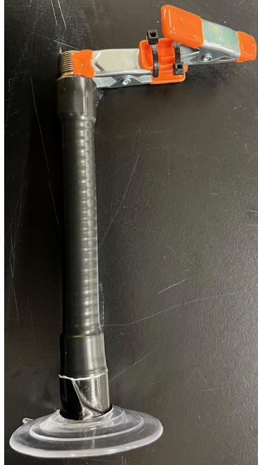
Figure H.8: Double spring clamps connected to the positioning arm and suction cup.
