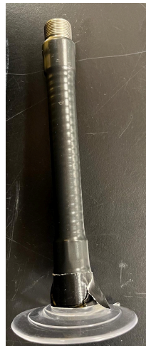
Figure H.7: The positing arm attached to the suction cup. The black tape is covering the excess adhesive from the bonding of the suction cup to the positioning arm.
