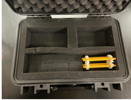
Figure H.11: Empty Pelican case with Pick and Pluck foam taken out of spots where components rest.
