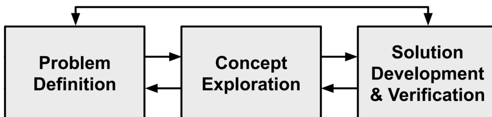
Figure 2. High-level schematic of our design process, obtained from the ME Capstone Design Process Framework [22]. The blocks shown specify the major design process steps encountered during the project timeline. Arrows signify the order of these steps, while reciprocated arrows between blocks show that iteration between those steps is expected.
