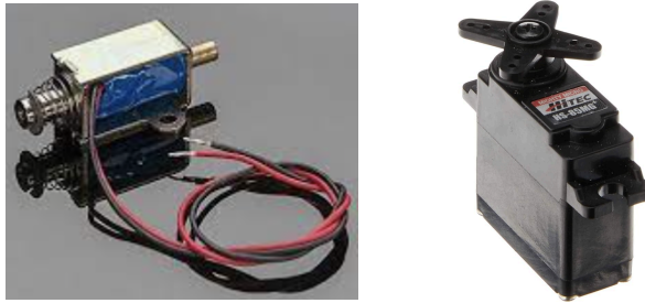
Figure 2. Push/pull solenoids (left) and servo motor (right)
