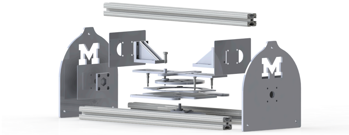
Figure 20. Exploded view of bellows system
