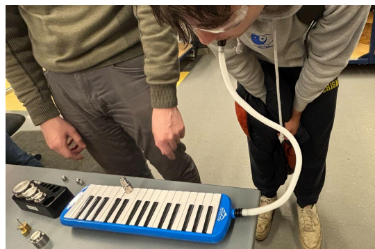
Figure 7: This image captures the key-press test in progress, where one team member would blow into the instrument while masses were stacked at the end of a key until it compressed far enough for a consistent note to play.
