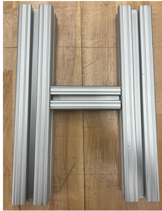
Figure 18. Figure 18 shows the final build for the Build the Track task. There are two of these sections on the board. There are four of the large sections that are 1.5x12x1.5” and two of the sort sections that are 1.5x3x1.5 ”.
