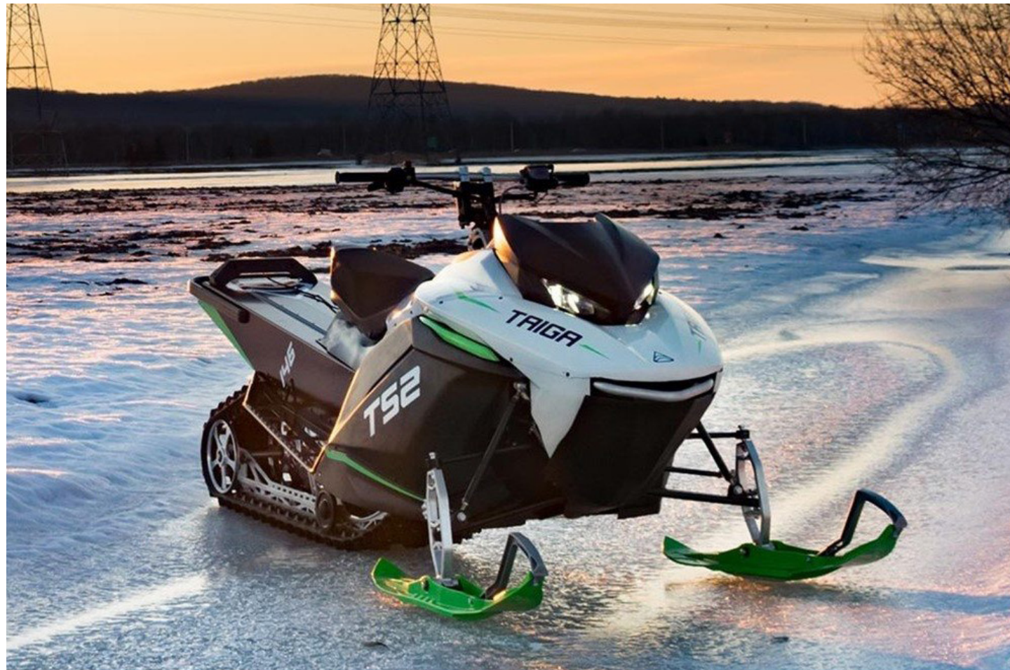
Figure 1.3: Taiga's EV snowmobile, the first electric model commercially available 2
