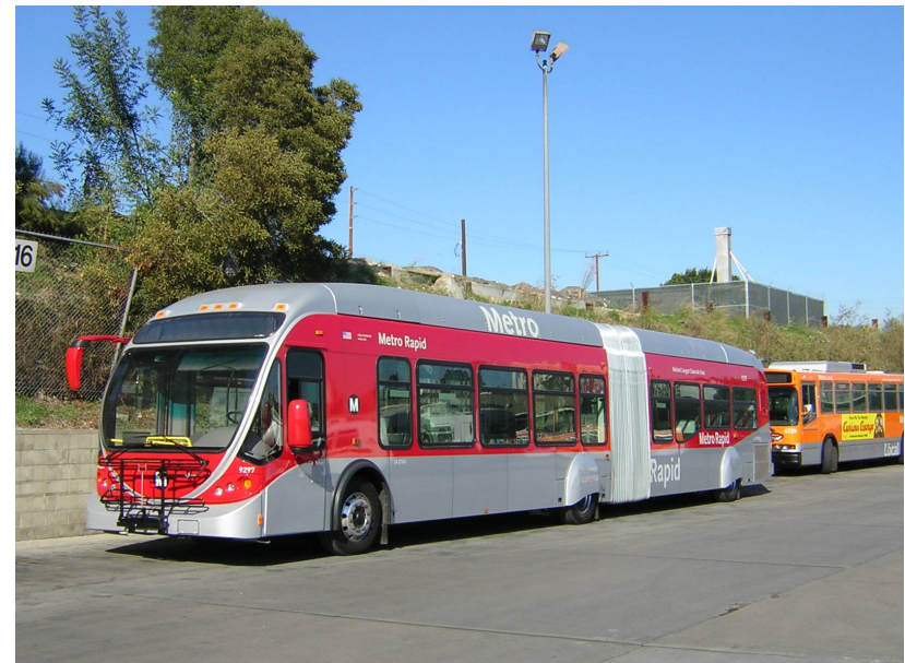
Figure 3.25: Metro Rapid Bus With Covered Wheels
