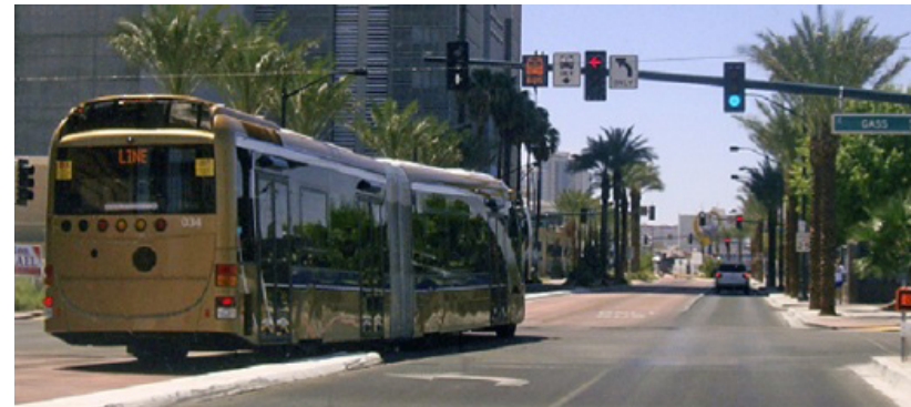
Figure 3.12: Las Vegas SDX Bus in Median Bus Only Lane
