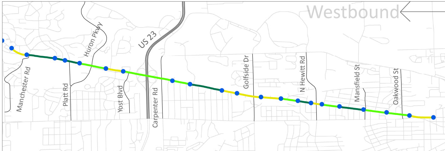
Figure 2.10: Off-peak Bus Speeds Between Stops on the Corridor (to Ann Arbor)
