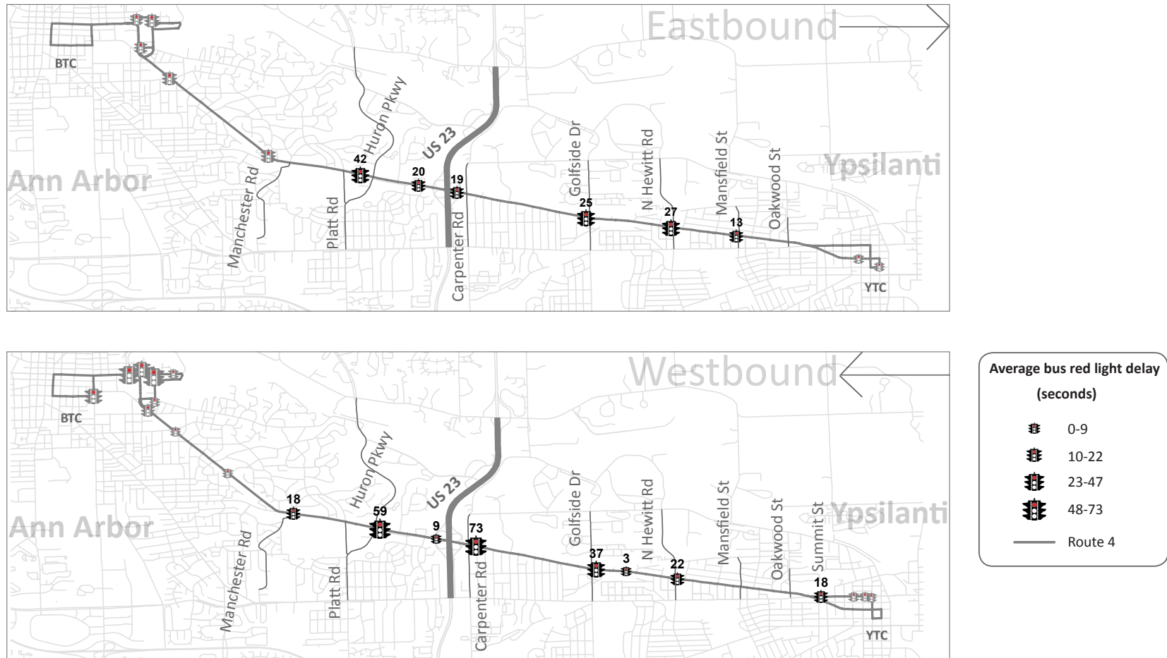
Figure 2.2: PM Peak Bus Traffic Light Delay on the Corridor
