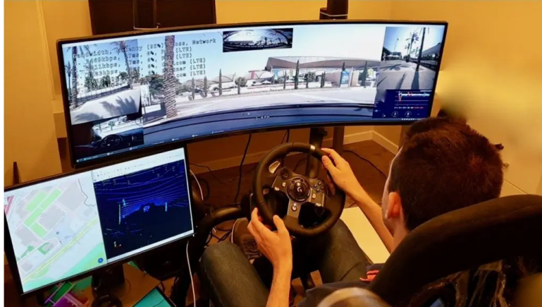
(a) Direct ToD: Human is driving remotely based on digital perception [131]
