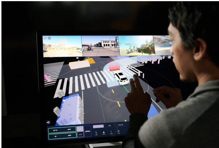
(b) Indirect ToD: AI recommends plausible paths for teleoperators to choose from [132]
