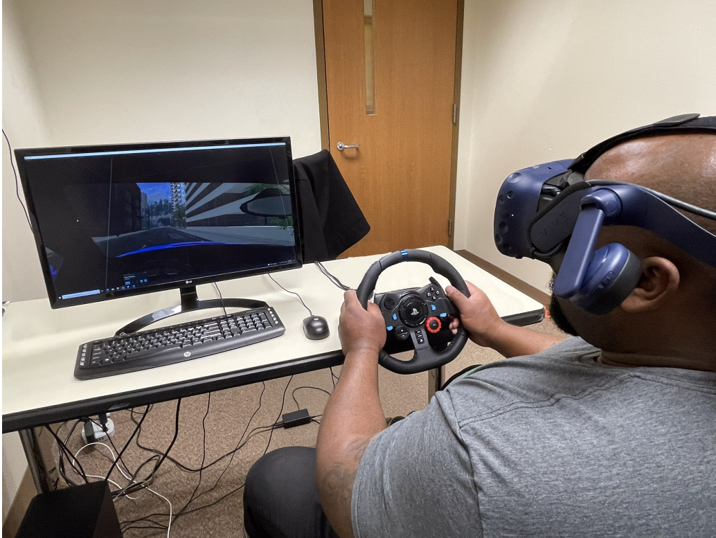
Figure 6.2: Experiment setup with VR driving simulator. Participant was wearing HTC Vive headset and driving a CV using Logitech G29 steering wheel and pedals. The screen shows the participant view in the VR environment.
