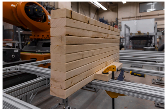
Fig. 9. The adaptive experimental scenario, with both robots alternating to assemble an NLT panel using the developed pose-based adaptive fabrication method.
