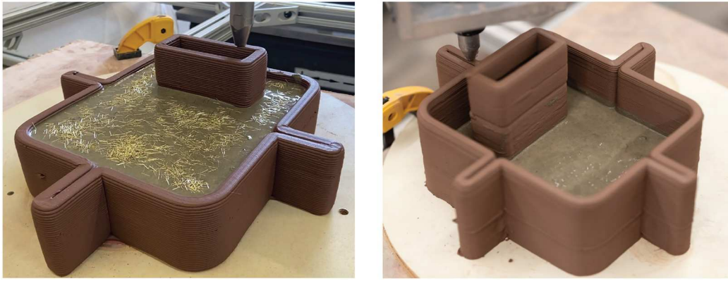
Figure 7. Formwork cross-section with four stiffeners and an internal void: interlayer (left) and mixed (right) fibers.
