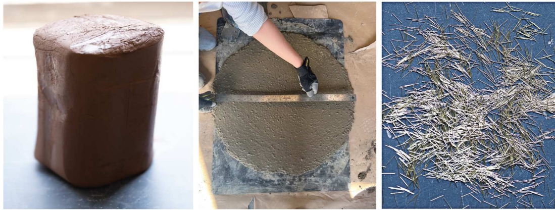
Figure 1. Commercial ready-to-use terracotta clay block (left), slump flow test of the SCC mix with a spread range of 500–600 mm (center), and steel fibers (right).
