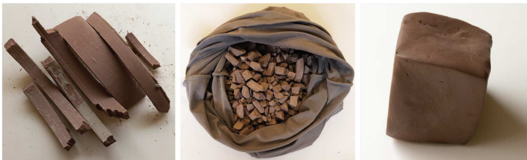
Figure 8. Recycling process: demolded formwork (left), crushed pieces in the fabric (center), kneaded clay ready for extrusion (right).
