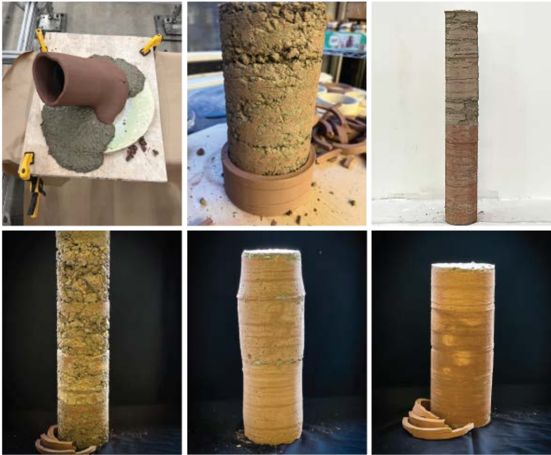
Figure 2. Sample trials to fine-tune the SCC mix, and adjust the retarder and accelerator proportions.
