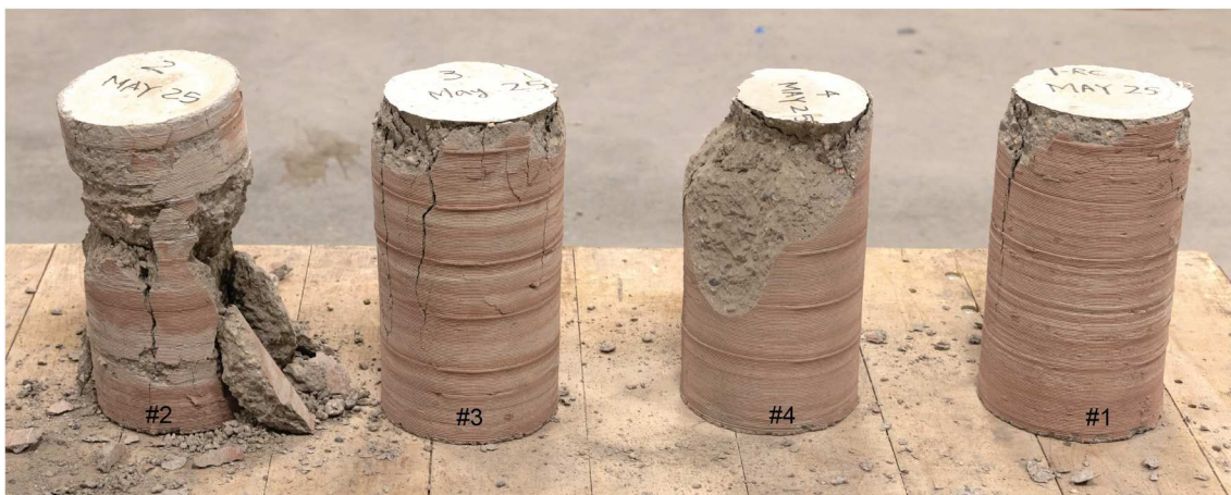
Figure 3. Cylinder samples used in the compression test; samples 2 and 4 showed lower compressive strengths.
