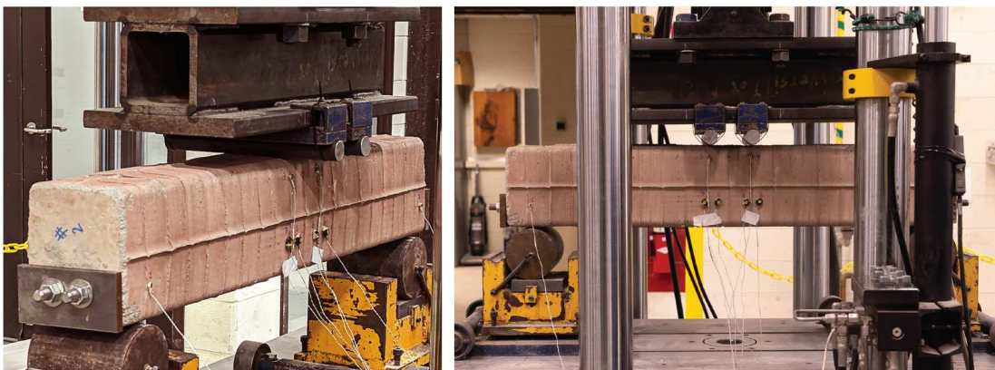
Figure 9. Four-point bending test setup with four pairs of kinematic tracking markers installed on the beam's surface.
