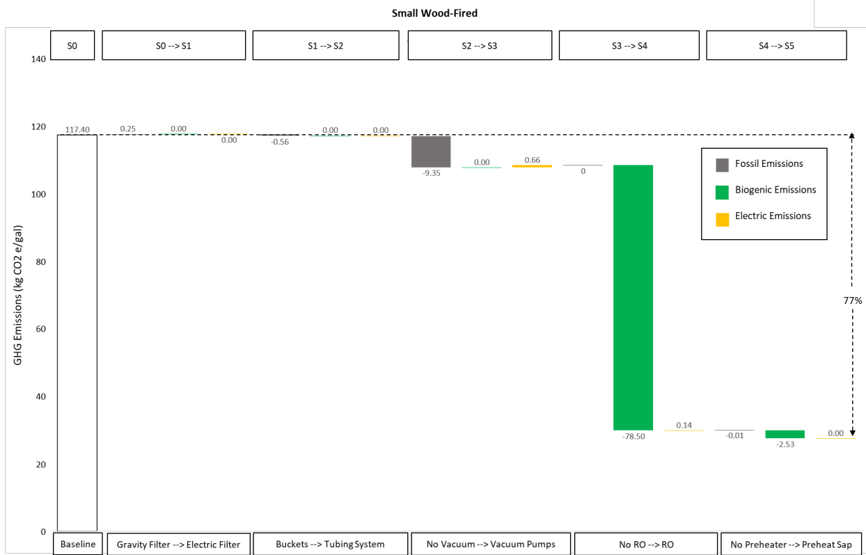
Figure 5 GHG emissions reduction by process change for small producers using wood as the evaporator fuel. Reductions for each emission type (fossil, biogenic, electric) are calculated with respect to the total emissions in the baseline case (gravity filtering, buckets, no vacuum, no RO, no preheater on the evaporator). All assume a 2022 syrup production weighted NAMSC average electric grid (0.18 kg/kWh), with the low end of the range being VT (0.02 and the high being WV (1.02 kg/kWh).
