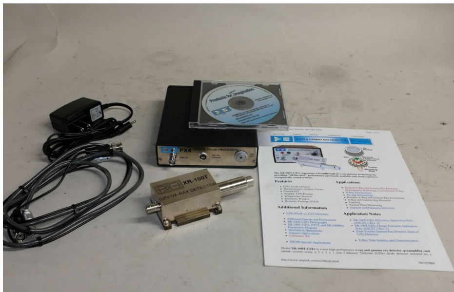
Figure 9.1: Amptek CdTe detector system designed for gamma ray measurements from 3 keV to \sim 150 keV. The detector preamplifier output is available and can be digitized by a CAEN digitizer or similar.
