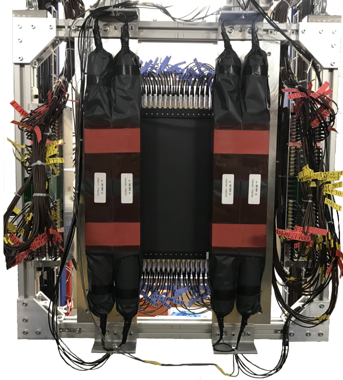
Figure 2.8: Photo of the beam monitor for MUSE.
