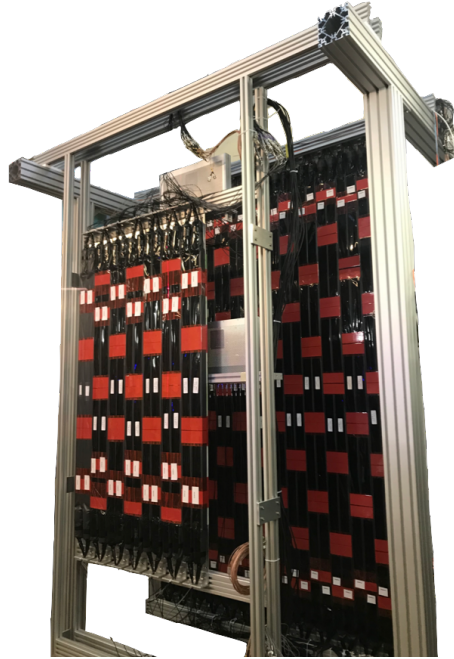
Figure 2.11: Photo of one set of walls of the SPS detector used for collecting timing and position information of scattered particles. Each side of the detector set up has two walls: a smaller front wall and a larger back wall.
