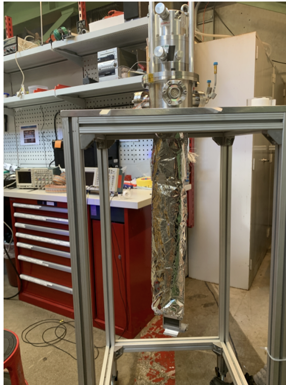
Figure 3.1: Photo of the target ladder wrapped in superinsulation before being craned into the vacuum chamber in PiM1 at PSI.
