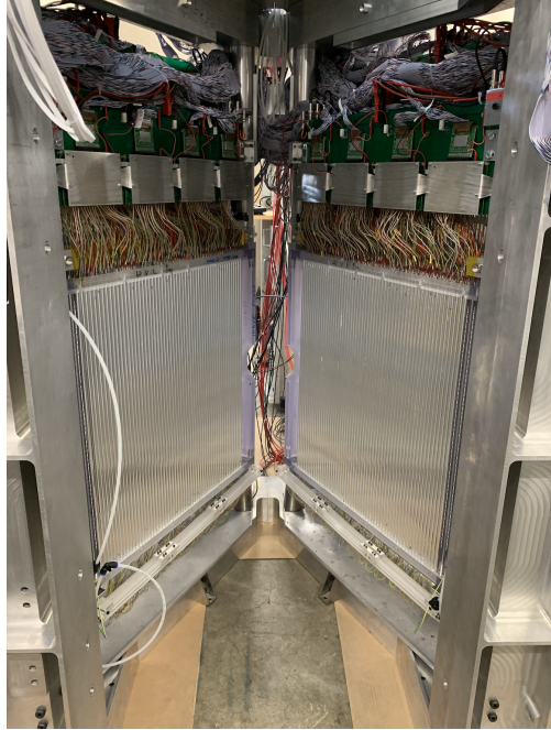
Figure 2.10: Photo of the STT detector while it is being repaired outside of the MUSE platform. The image is looking in the beam direction, and the straws shown are closest to the vacuum chamber in the detector set up.
