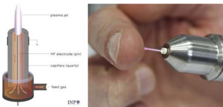
Figure 1.9. Schematic and example use of the kINPen. Adapted from [26].
