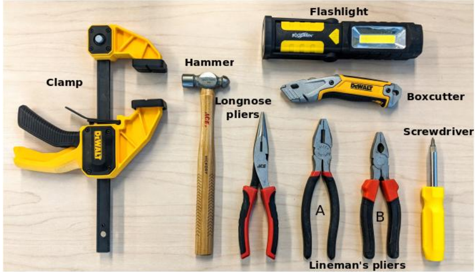
Figure 3.4: Objects in our custom dataset. The clamp has one prismatic joint. The three sets of pliers each have one revolute joint. The other four objects are treated as rigid. The objects are separated into parts based on the presence of both affordances and articulations.
