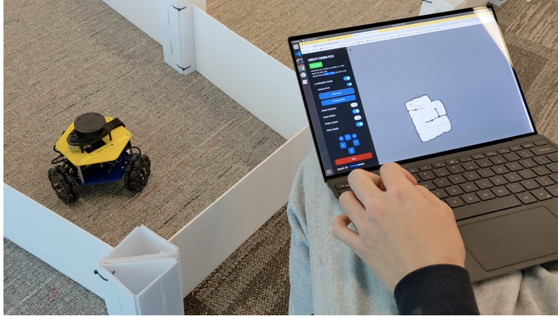
Figure 6.5: The MBot Web App in action. The web app can be accessed through a browser on any device connected to the robot’s network, and enables teleoperation of the robot, control over the SLAM state, and visualization.
