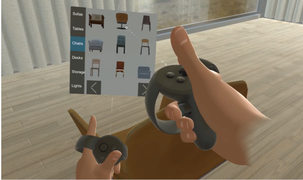
Figure 5.1: The immersive authoring environment. A menu is always attached to the left controller. Users can select pre-made furniture models of different categories and place them in the VR scene.
