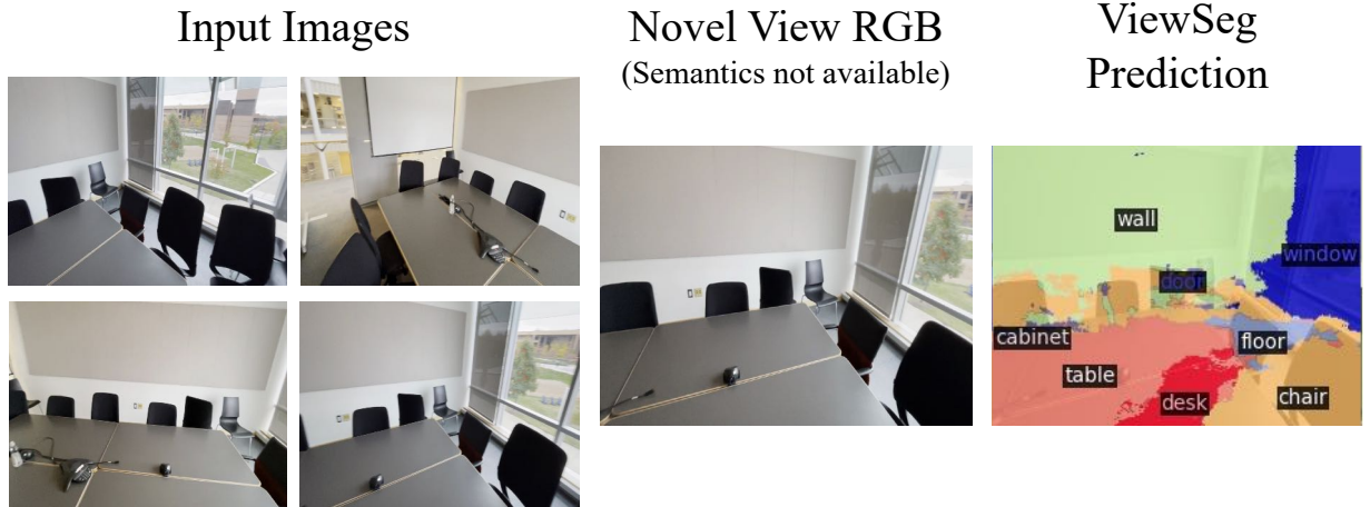
Figure 3.5: We test on real images taken with an iPhone 12. Despite noisy camera poses estimated by COLMAP [234] following [189], ViewSeg obtains reasonable segmentation results.
