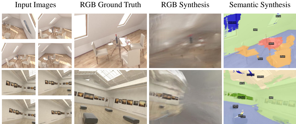
Figure 3.2: RGB is a poor bottleneck representation for semantic synthesis. While one may be certain of the labels of the new view (e.g., walls, tables), synthesizing the particular wall or table pixels from few views is challenging: outputs are often blurry (top) or collapse when extrapolating (bottom).
