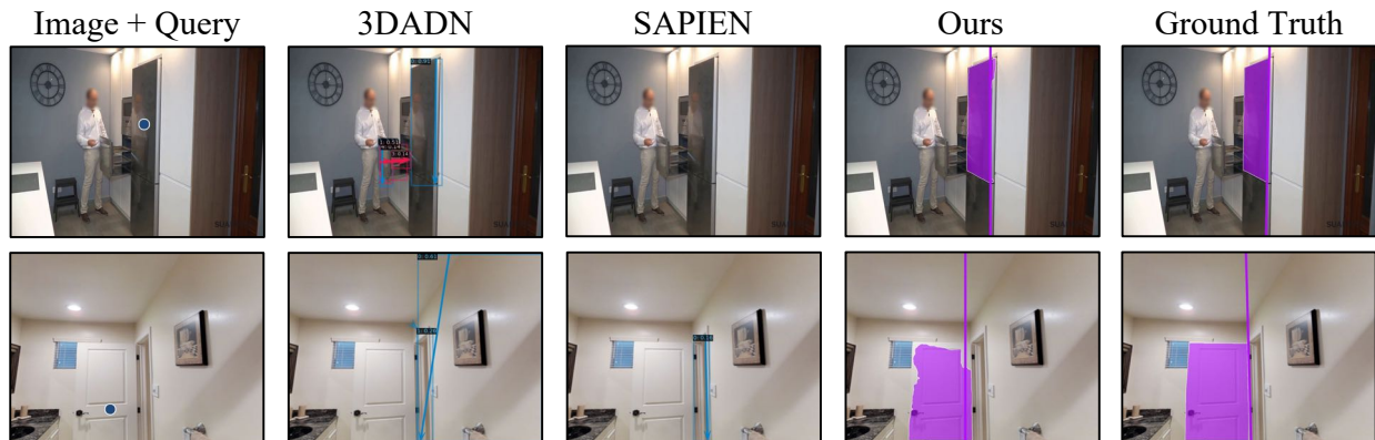
Figure 5.6: Comparison of 3DADN [211], SAPIEN [287] and our approach. 3DADN has a strong performance when humans are present. However, it has difficulty detecting objects without human activities. SAPIEN does not generalize well to real images. However, it is sometimes better than 3DADN when humans are not present.
