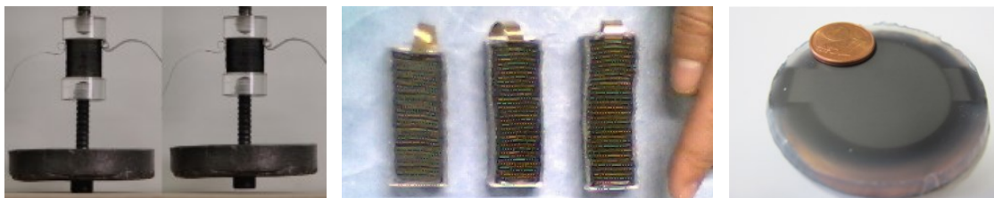
Figure 6. Dielectric Elastomer Actuators with Frameless Configurations.
