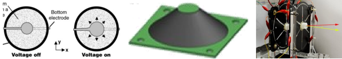
Figure 7. Dielectric Elastomer Actuators with Rigid Frame Configuration.
