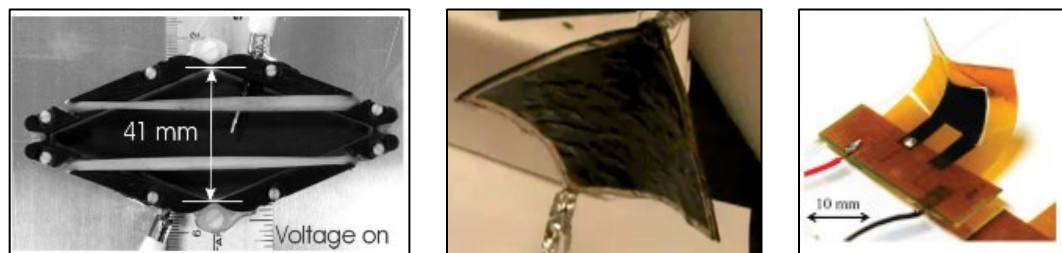
Figure 8. Dielectric Elastomer Actuators with Flexible Frame Configuration.
