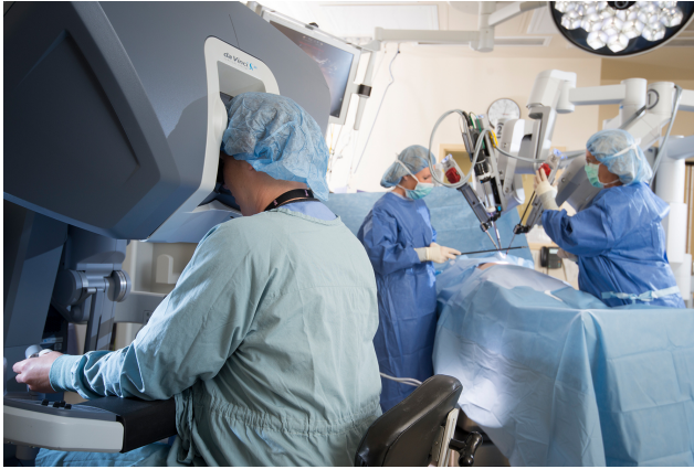
Fig. 3. The Da Vinci Robotic-Assisted Surgery System, that participant Dr. Nabeel Shakir uses to perform gender-affirming surgery procedures. The system involves an extended reality headset and hand controls that enable the surgeon to perform the surgery “remotely” from elsewhere in the same room. image info: “Robot assisted surgery,” licensed under Creative Commons Attribution-Share Alike 4.0 International .
