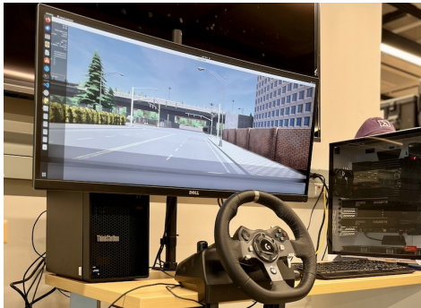
Fig. 5. The simulator used in the pilot human subject study. The throttle/brake pedals are on the floor.
