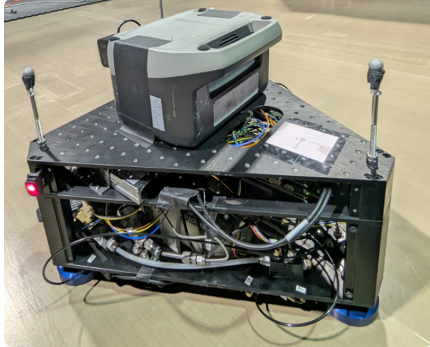
Fig. 4 The air bearing sled on JPL’s GSAT flat floor facility used for hardware verification, with +y pointing toward the right.
