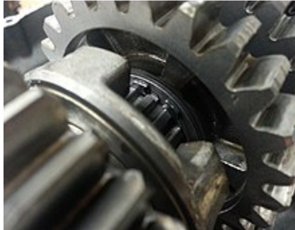
Figure 3.1.4 Honda CBR1000 Dog Gears
