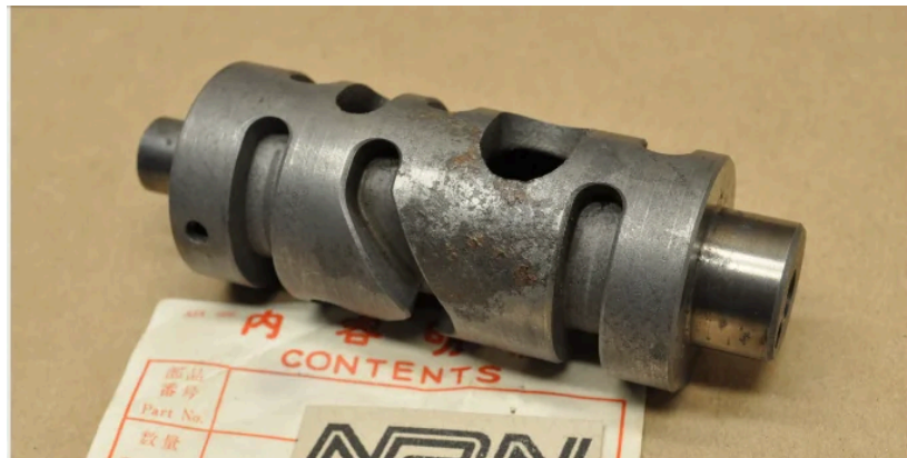
Figure 3.1.5 Honda Recon 2x4 Transmission Selector Drum
