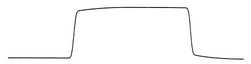
Transmitted Pulse: Maximum Magnitude = 6.68E-01 Total Transmitted Energy = 6.63E-01
