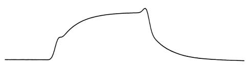
Transmitted Pulse : Maximum Magnitude = 3.12E-01 Total Transmitted Energy = 2.89E-01
