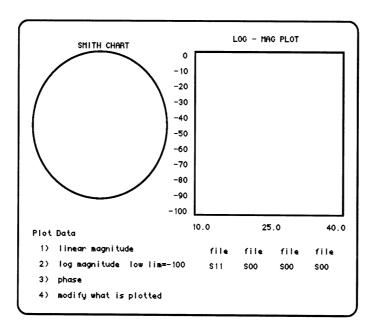
The rectangular plot x-axis is always frequency, with the limits being the start and stop frequencies. The options and their functions are:
