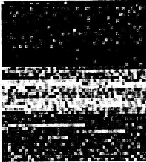
Figure 3.12: A profilometer scan showing the level shifts. (The EDM did not move during this scan.)
