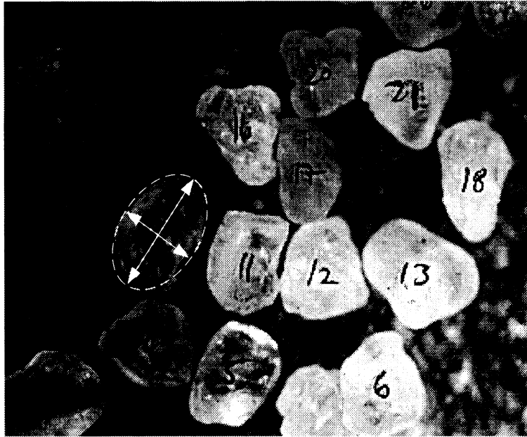
Figure 2.6: Determination of particle grain size distributions, modeled as prolate ellipsoids. Each grain was modeled as an ellipsoid
