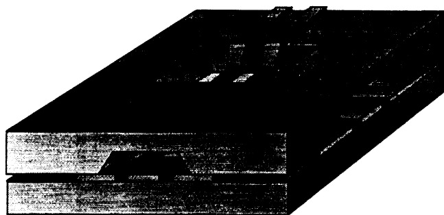
Fig. 5.2: Si micromachined two-layer packaged circuit. The upper wafer shields conductors and provides support for vertical integration.
