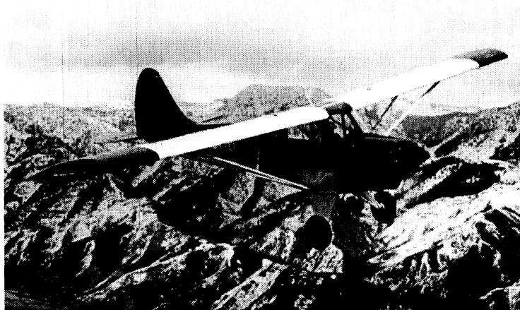
Figure 3. Aviat Husky A1-B. As the current equivalent to the venerable Piper Super Cub, this aircraft serves as our design baseline for STAR-Light.
