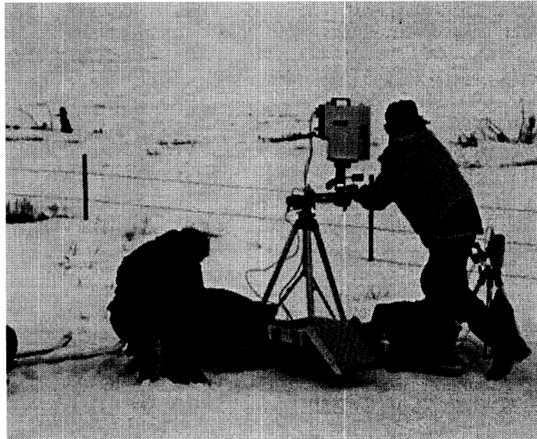
Figure 6.21: Operator holding reference panel under spectroradiometer for reflectance measurement
