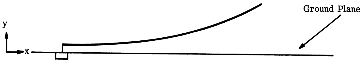
FIG. 2-2: GEOMETRICAL REPRESENTATION OF AN ASYMMETRICAL RUDIMENTARY HORN.
