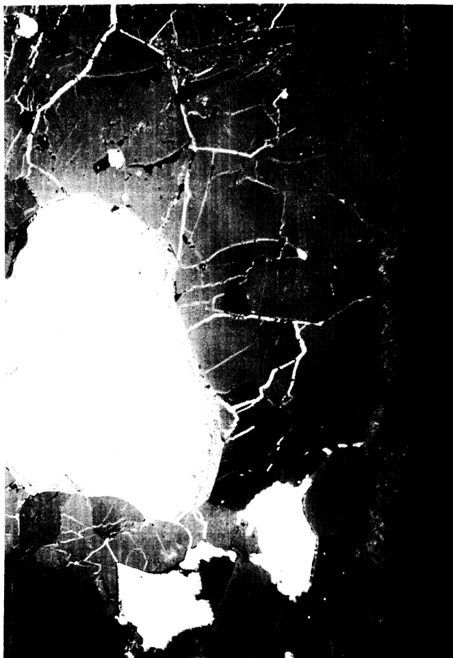
FIGURE 19: FUSION CRUST ON MODOC. THE BLACK RIM ALONG THE OUTER EDGE OF THE CRUST AT RIGHT IS CAUSED BY ROUNDING OF THE EDGE DURING POLISHING. OUTER ZONE OF CRUST IS HERE ABOUT THE SAME WIDTH AS THIS BLACK RIM. THE WHITE GRAIN NEAR BOTTOM EDGE OF PHOTO IS SULPHIDE; OTHERS ARE NICKEL-IRON. THE VEINS ARE SULPHIDE. THE OUTER EDGE OF THE LARGEST GRAIN HAS A RIM OF SULPHIDE (NOT EASILY SEEN IN THE PHOTO) WHICH IS PARTIALLY REPLACED BY LIGHT GRAY HYDRATED OXIDE. ( \times 250 ).
