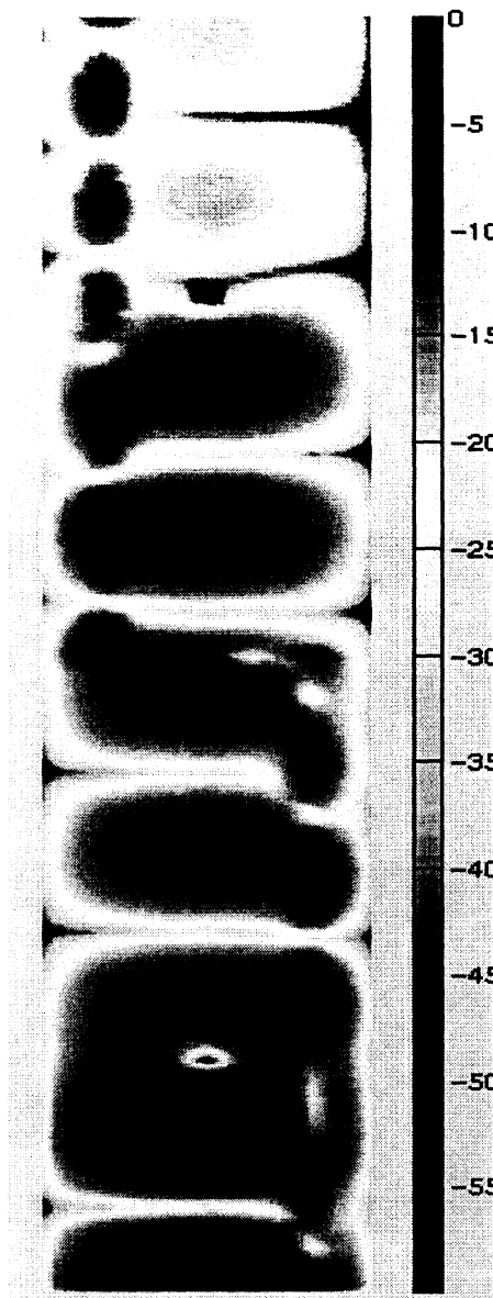
Figure 47: Field Distribution for the cavity with bended striplines case II-G. ( f = 1.44f_c^{TE_{10}} , \Delta h = 56.76 h )
