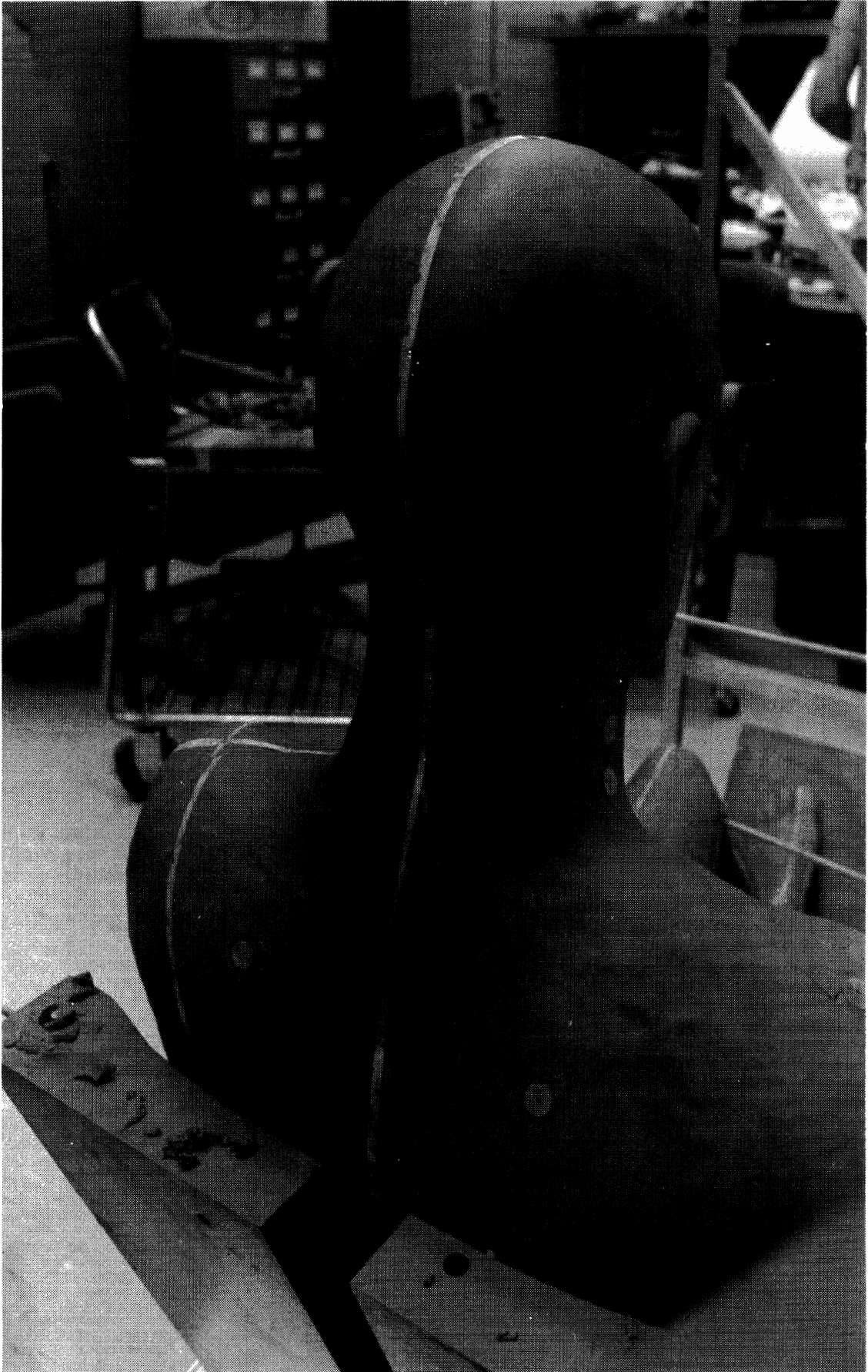
FIGURE 10. Back view of clay model with surface profile strips.
