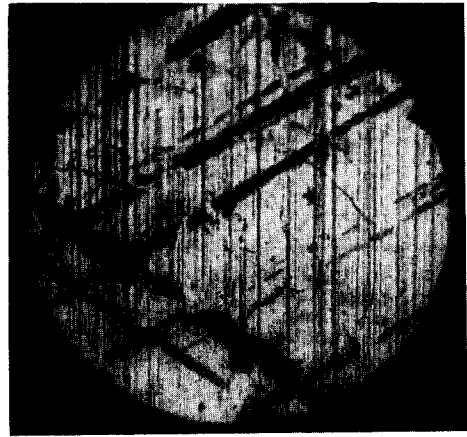
Fig. 20. Run for 15 h. Location shown is at the TDC position of the top ring (magnification 202 \times ).
