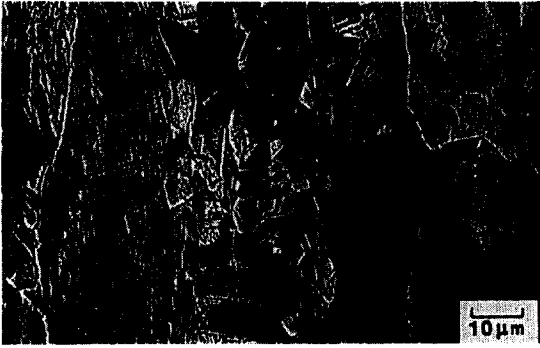
Fig. 1. Microstructure of copper uniaxially compressed 179% and partially recrystallized by annealing for 3 h at 200°C, showing nonhomogeneous distribution of recrystallized grains. Image obtained under channeling contrast conditions in a scanning electron microscope.
