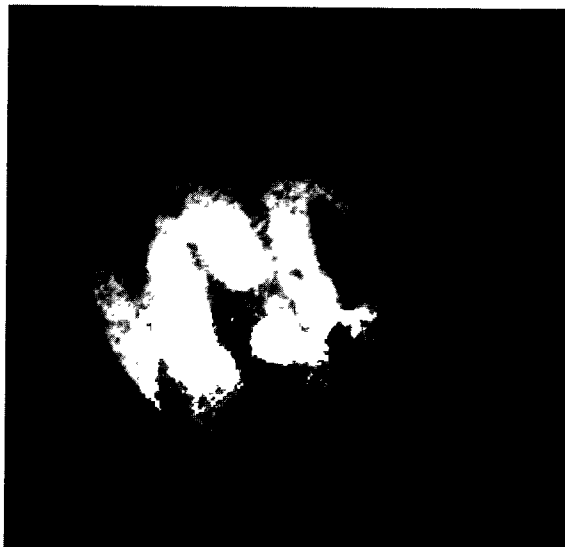
Fig. 1. A PRM image of a 25 \mu\text{m} thick Mo foil that was annealed for one hour at 1800 ^{\circ}\text{C} . The area imaged is approximately 500 \mu\text{m} on a side; the magnification is 22 \times ; and the resolution is 2 \mu\text{m} . The image presumably depicts crystalline domain growth or possibly patches of impurities that have segregated at the surface.
