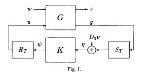
In Figure 1, since u is the output of a (zero-order) hold operator as given in (5) it follows that
