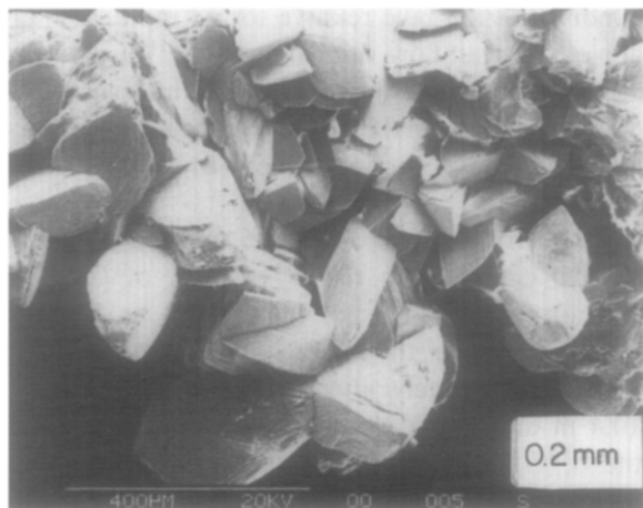
Fig.13. Scalenohedral calcite crystals cemented in fine-grained calcite crusts from 4.4 m in WLC84-8.
