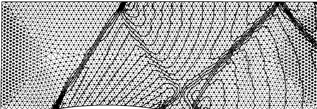
Fig. 2. Supersonic channel flow with an inlet Mach number of 1.4. Iso/Mach lines with increment 0.05, superimposed on the mesh (1977 vertices). Wave model C, NN scheme.
