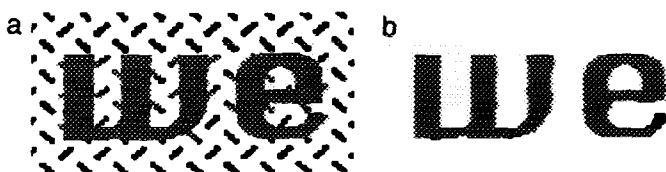
FIG. 4. (a) The word "we" with a uniform background. (b) Background removal after opening the image with a 9 \times 9 square structuring element.
