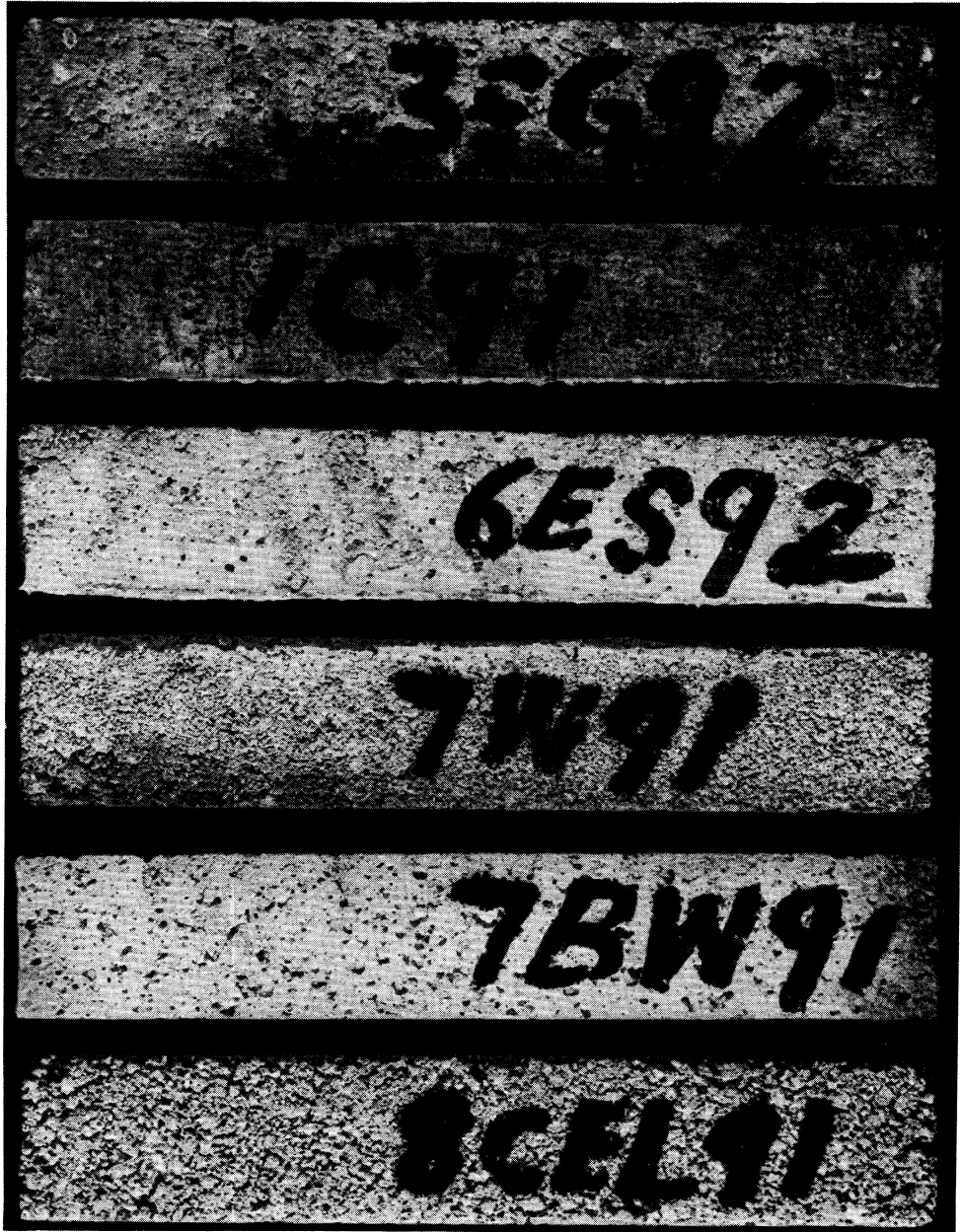
Figure 11. Concrete Specimens After Staining and Popouts Test.
