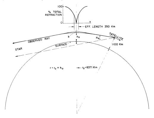
The figure illustrates the experiment in the case of the earth with  $R_n$ ,  $h_o$  and b exaggerated. The small upper figure shows per cent of total refraction as a function of horizontal distance x to illustrate the effective length of the probe. Dimension b, given by
