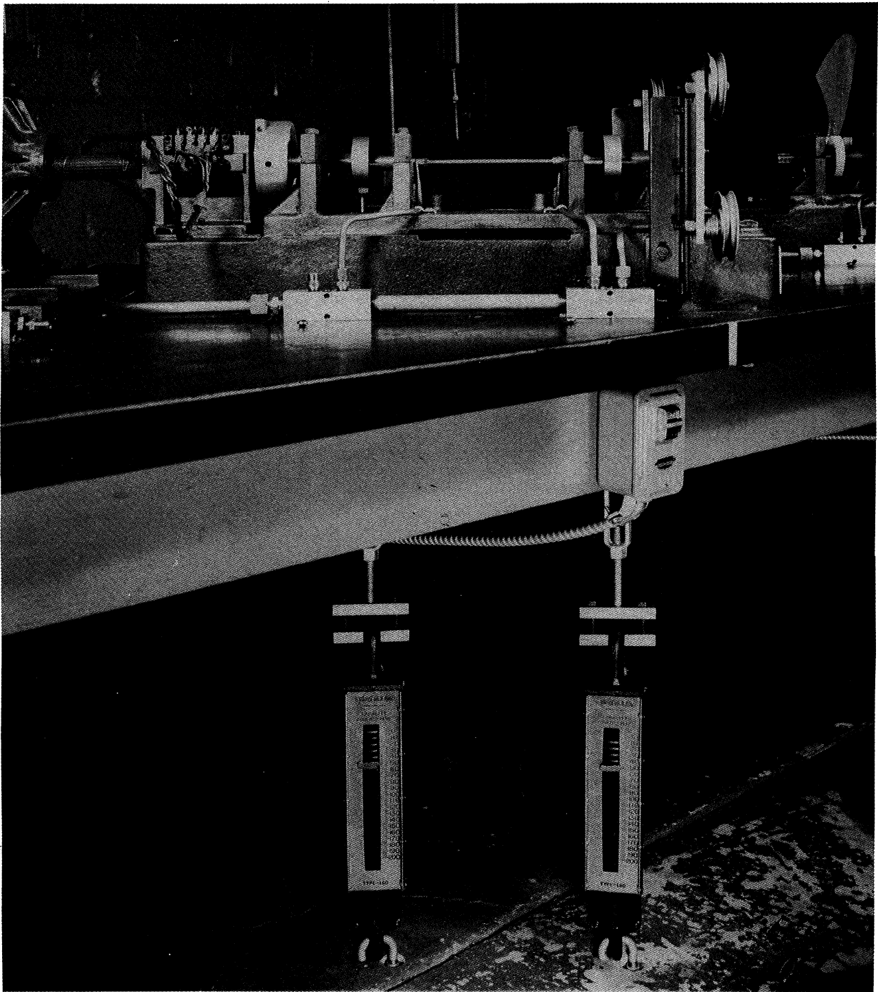
Fig. 10. Bearing-friction test set-up.
