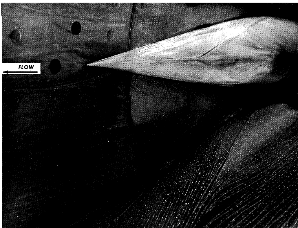
Fig. 5. Boundary-layer streamlines with inserts No. 1 in highest Mach number position in U. of M. 2.84 nozzle.
