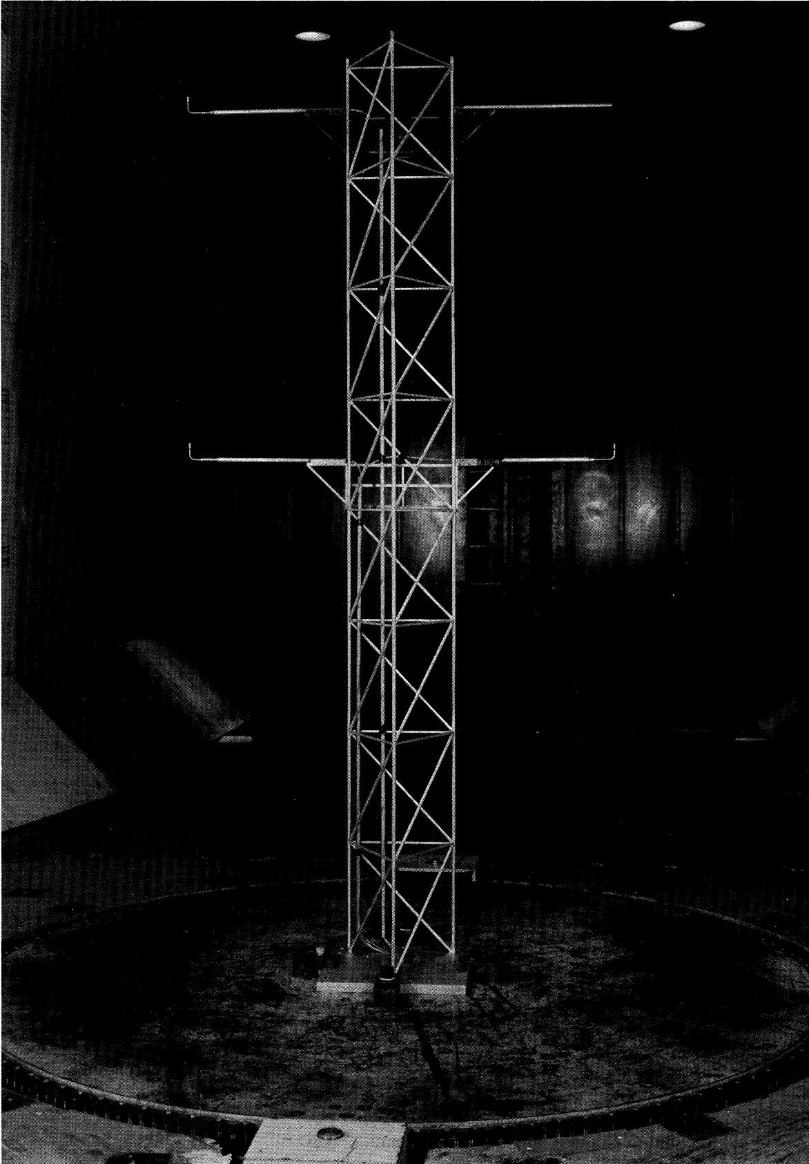
Figure 7. Section of 1/8-scale Model of Kennedy Space Center Meteorological Tower with Three Probes in Place. Tower section is in test position in sixteen- by sixteen-foot Langley Transonic Dynamics Wind Tunnel.
