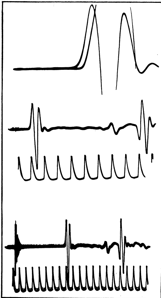
FIGURE 6. OSCILLOSCOPE TRACES FOR V_p MEASUREMENTS ON NIPISSING DIABASE AT 8 kb. The lowest photograph shows microsecond timing marks on the trace; on the other, reading from the left, can be seen the electrical pickup from the pulse, the first arrival, PSP, and a reflection of P from the outer end of the backing piece. The middle photograph shows the same pulse as the lower one with a faster sweep, the pulse now displaced from the screen. The top photograph shows the same pulse again, with still faster sweep; only the first arrival with the Hg signal slightly displaced from coincidence is shown [33].
