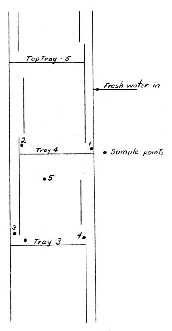
Weir height 31/2 in. Splash Boffle: 4 in from tray, I in from weir
