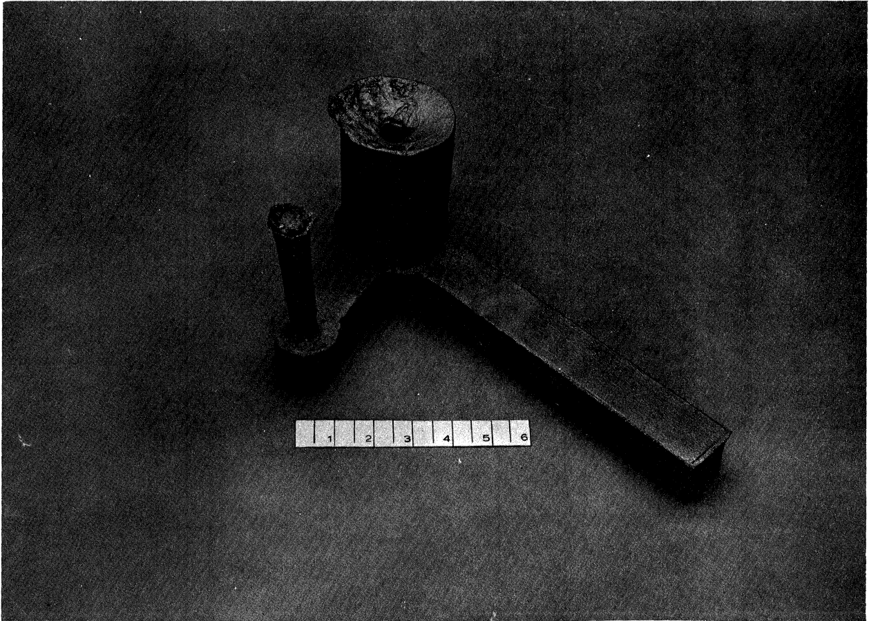
Figure 5. 1-1/2" x 1-1/2" x 10" end chilled bar. Gating and risering were similar to that used in the standard 2" x 2" x 12" castability bar (thermal gradient investigation).
