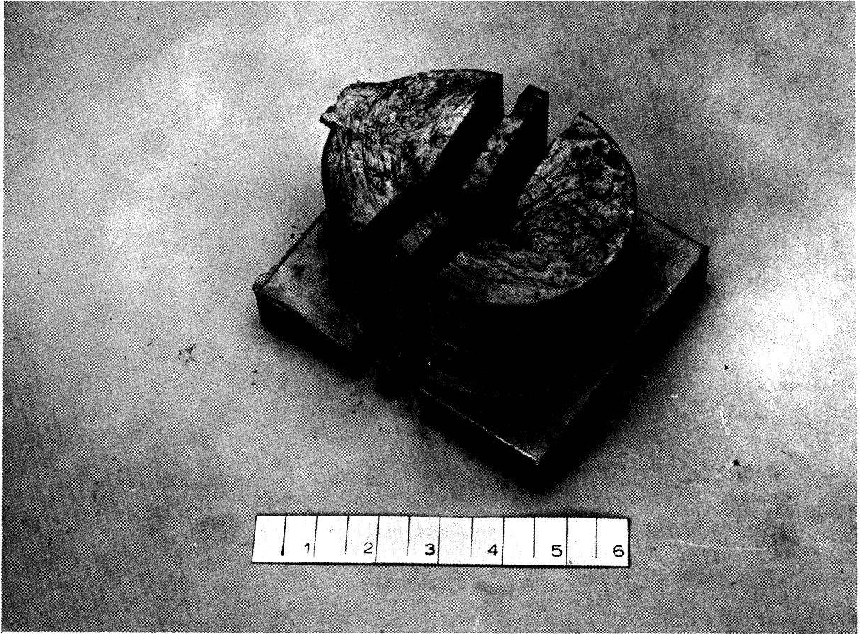
Figure 1. Plate casting with a large top riser which shows the slice used for radiographic examination.
