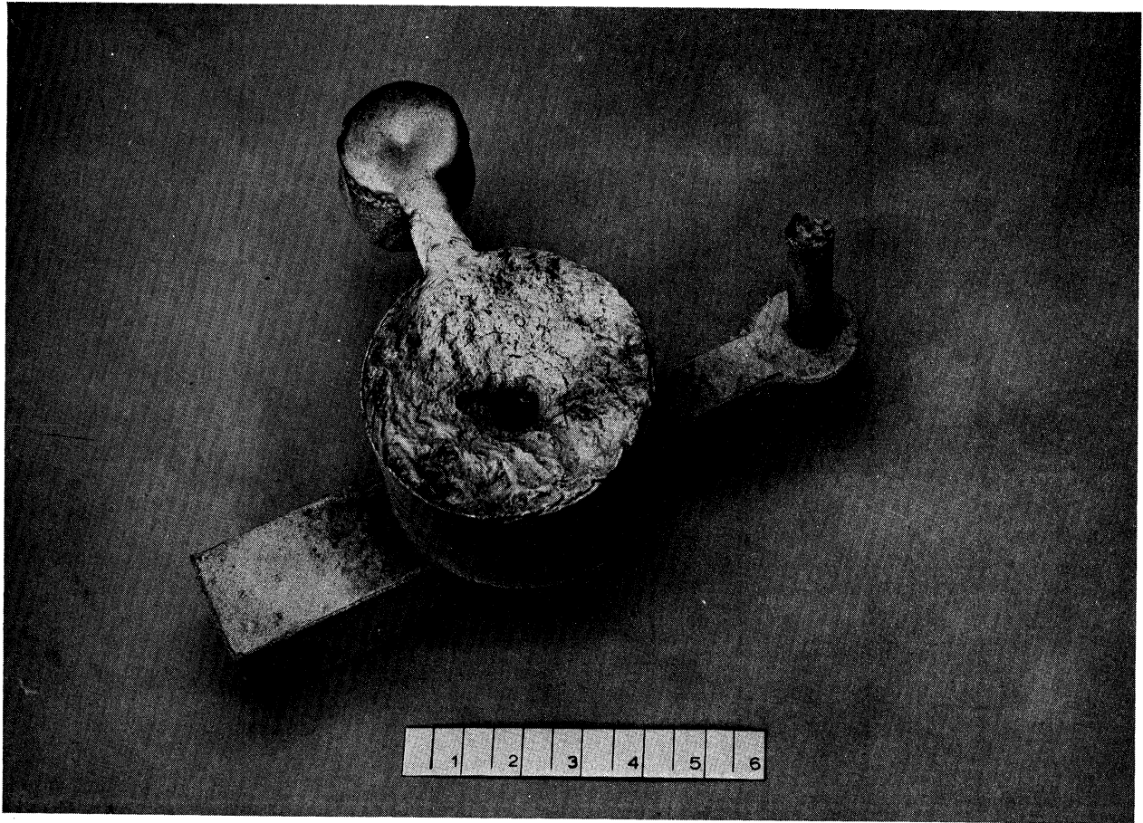
Figure 26. Top risered bar which shows the flow-off channel used to maintain a constant (H/D) ratio for the riser.
