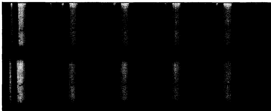
Fig. 3. Sedimentation pattern of erythrocyte cytochrome b_5 . The protein (2.3 mg/ml) was subjected to ultracentrifugation at 20 °C and 59780 rev./min in 0.1 M Tris-HCl buffer containing 0.5 mM EDTA, pH 8.1. Photographs were taken at 4-min intervals after 2/3 speed was reached.
