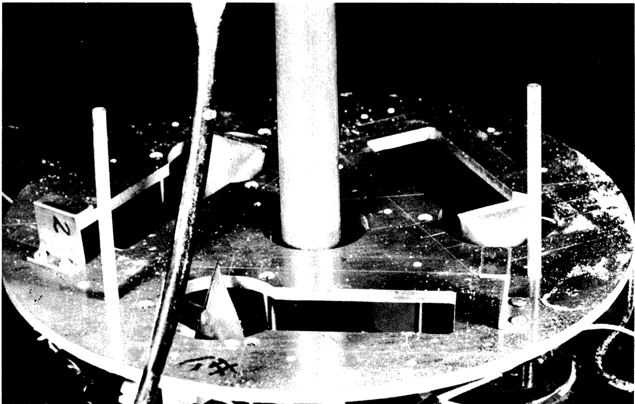
Fig. 6. Cold Weld Seals Made in Flight, SC-17
